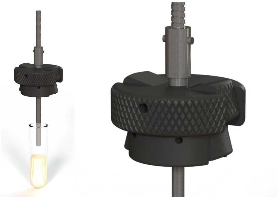
Figure 3: Sample Vial Holder and Glass Sample Vial [Inset showing clamps depressed]
